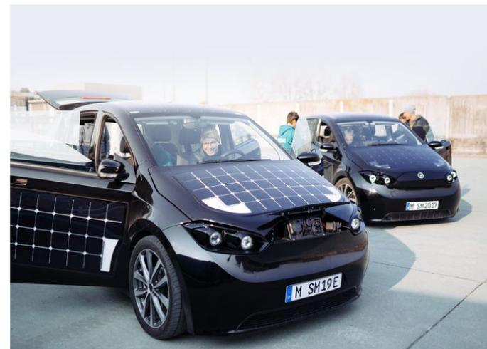
Figure 4: The Sion (Sono Motors) with 1.2 kWp of solar cells integrated in the car body.
