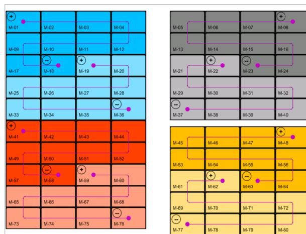
Figure 1: The stringplan of the PV plant.
