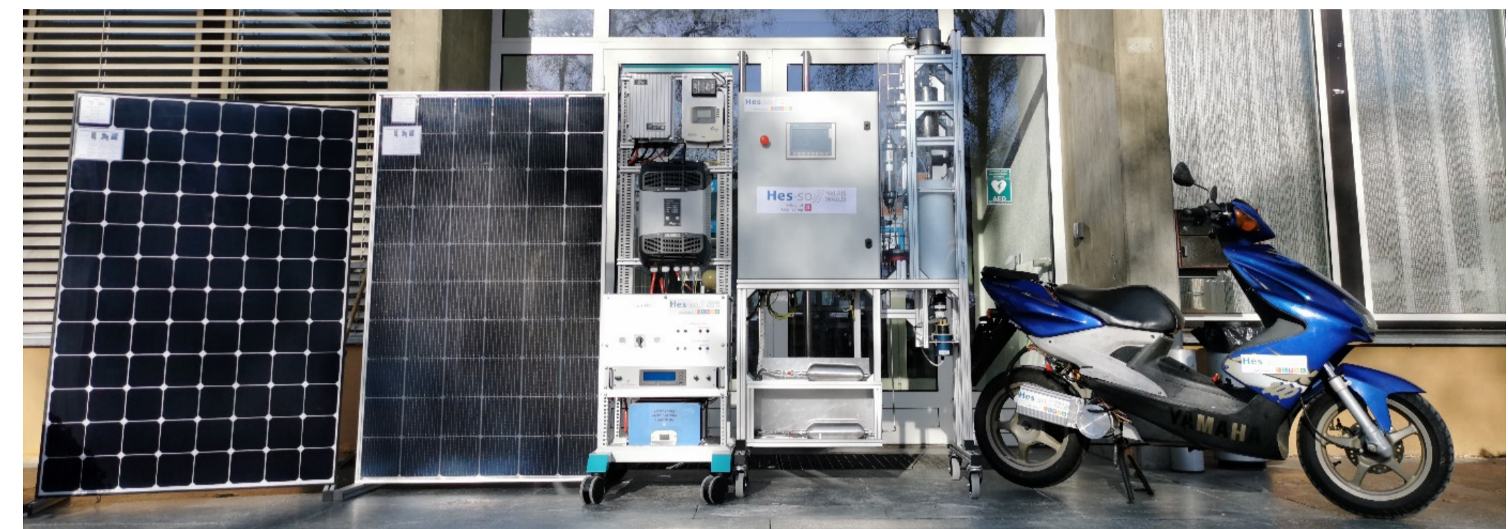
Using hydrogen to transmit solar energy to the wheels of a converted scooter
