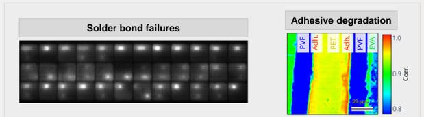
**Solder bond failures:** Recurring solder bond cracking caused increased series resistance and fill factor loss in SM55/AM55 modules, highlighting manufacturing quality issues.
