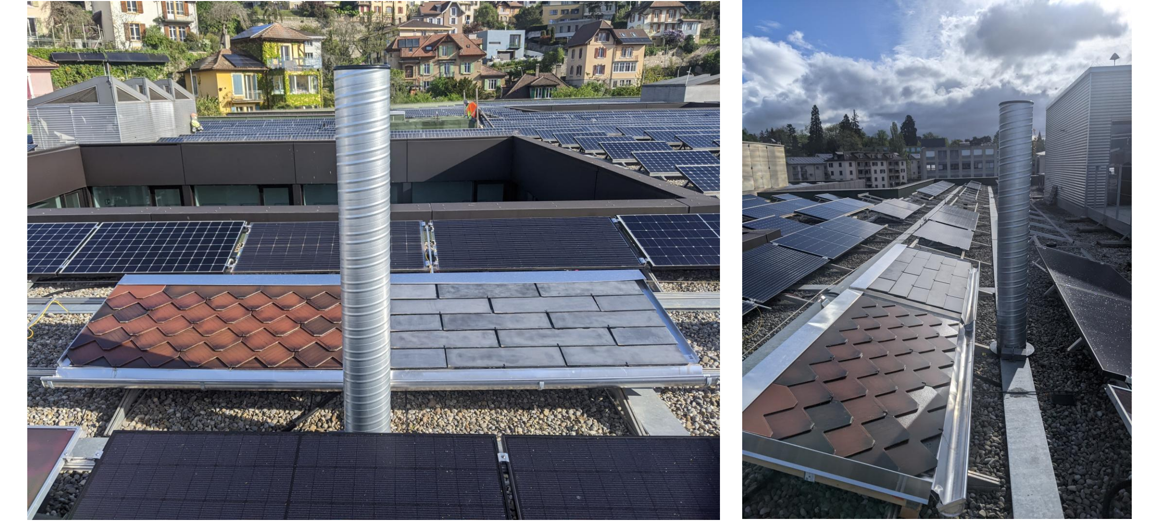
Fig. 4: Obstacle installed in front of monitored outdoor roof tile modules
