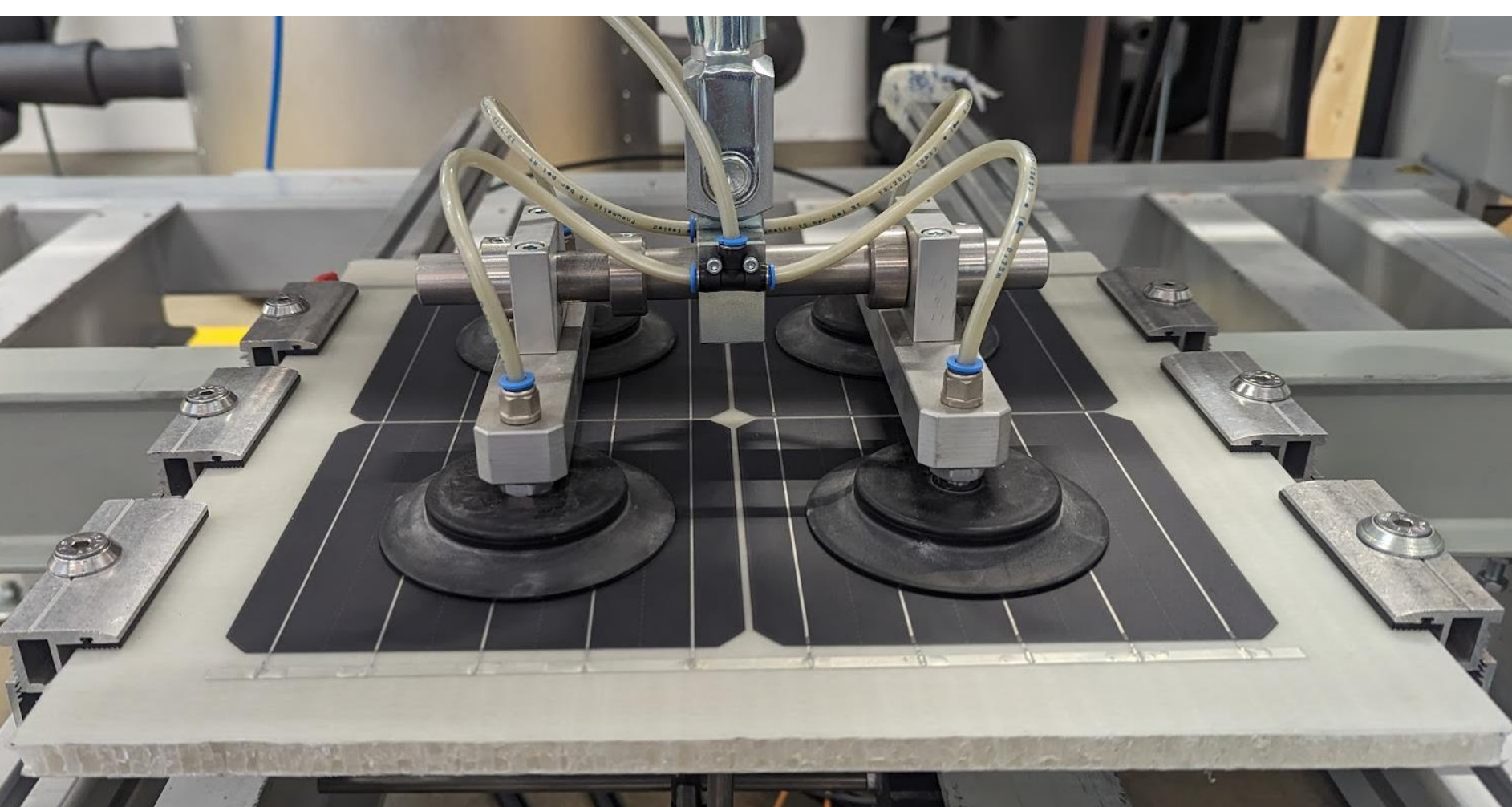
Fig. 8: Mounting of a 4-cell PV module for Mechanical loading consisting of three cycles of ±2400 Pa
